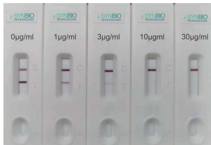
Test card color rendering display diagram
